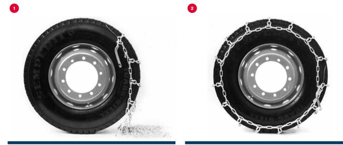
Hang the chain into the tire thread by means of the enclosed mounting cable.
